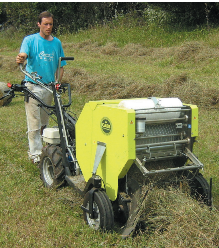
Walk-behind tractor with round hay-baler implement.
