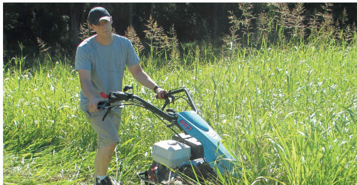
Walk-behind tractor with 59-inch sickle-bar mower.
